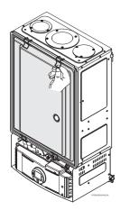
Fig. 5 Remove the combustion cover
